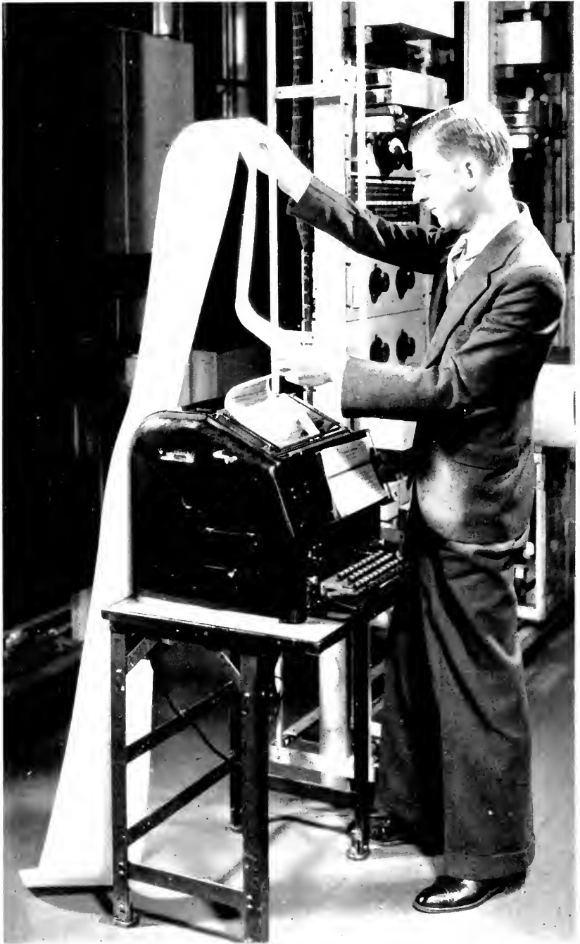
FIGURE 2. ONE DAY'S PROGRAM ORDER, 15 FEET LONG, SENT BY TELETYPEWRITER FROM NEW YORK TO ALL TELEPHONE COMPANY OFFICES INVOLVED IN FURNISHING NETWORK SERVICE.
